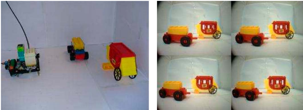
Figure 19. Tiny Lego Robot performs relative distance estimation by utilizing peering method. Sequence order: top left, top right, bottom left, bottom right.
