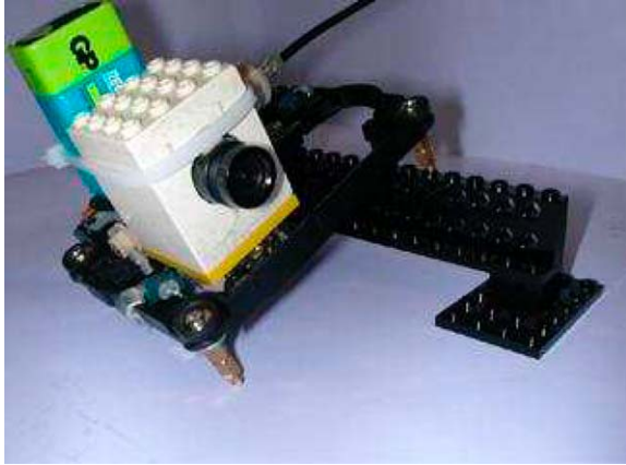
Figure 22. Scheme of the implementation of the miniature Mantis Head camera platform, which utilizes the diagonal peering behavior for distance estimation.
